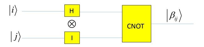
A gate based circuit for generating a Bell state
